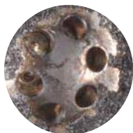
Injector after one P.i. treatment.
